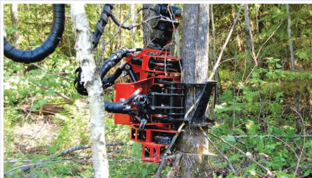
This is a giant leap forward in professional energy- and small wood harvesting. With this unique head you cut small bushes, twigs and thinner trees with a snap and fell bigger trees using the saw. The head also works perfectly as a traditional loading grapple. The XG220 is a combination of two of the most successful and tried out Mecanil products; Mecanil EG250 energy wood felling head and SG220 grapple saw. The head is very easy to install because of no need for any additional hydraulics.
