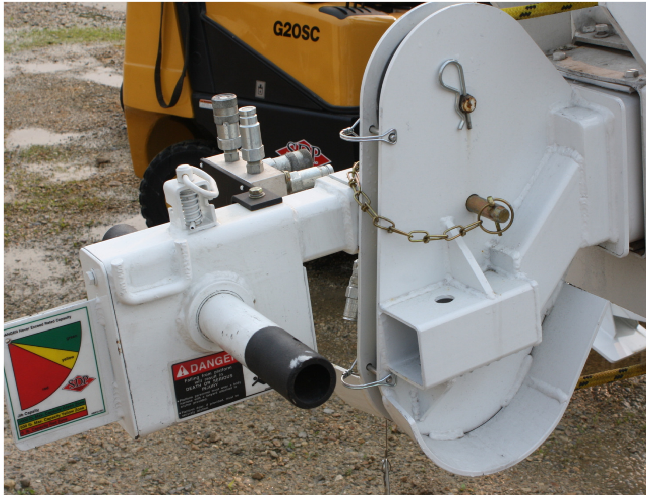
Shows the bucket mount installed and pinned in place
