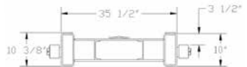
HOIST FRAME DETAIL
